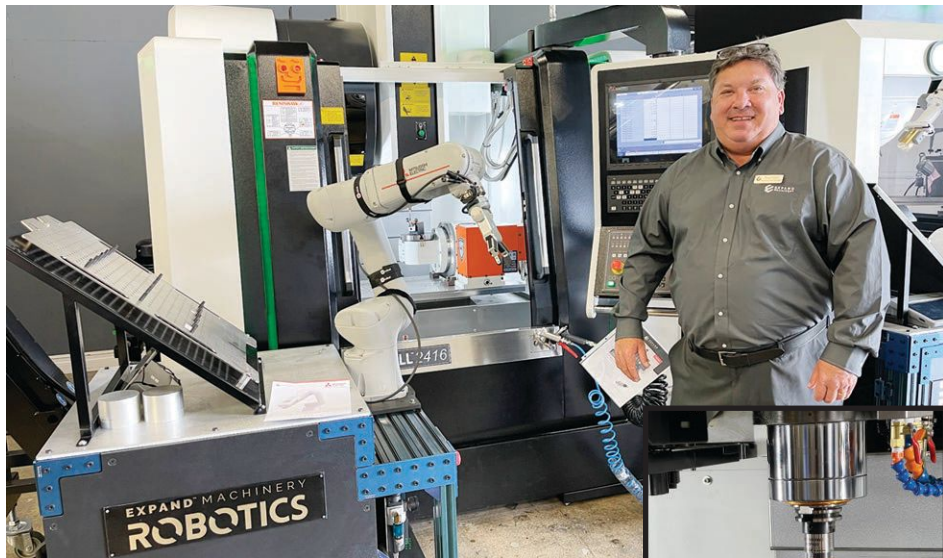
Doug Henke, Regional Sales Manager, Expand Machinery, with the GEN MILL 2416 3-axis high-speed VMC with 24-tool high-speed double arm ATC; 1,417 IPM rapids; spindle chiller and 12,000 RPM double-ground BIG-PLUS spindle. It features the Mitsubishi RV5 Assista Cobot with a 3-year warranty for both the control and robot.
