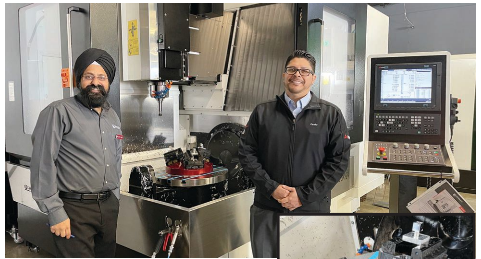
(l-r): Ravjeet Singh, General Manager, Expand Machinery and David Contreras, Business Development Manager, Machine Tool, Mitsubishi Electric Automation, with the GEN MILL 5X-24 CNC milling machine. The machine features a 25.6" worm-gear driven tilting rotary table and precision glass scale feedback in the XYZ axes as well as the rotary B and C axes.
