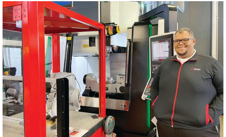
Henry Gomez, Senior Field Application Engineer, Mitsubishi Electric Automation, with the 5X-12 GEN MILL high-speed VMC with built-in 12" trunnion with glass scale feedback on all 5 axes; roller bearing ways; 1,417 IPM rapids; 12,000 RPM double-ground BIG-PLUS spindle and spindle chiller. It features the Mitsubishi RV20 FR LoadMate machine tending robotic cell with zero-point workholding.
